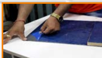
Step 1 : Remove the protective film from the SURFACE of the side which has to be PASTED.
