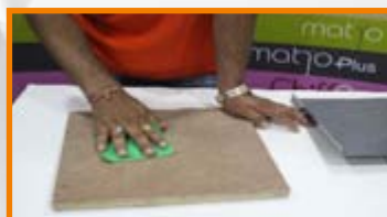
Step 5 : Also SCRATCH plywood Surface
