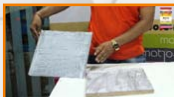
Step 9 : BERGA PVC GLUE to be applied to both the SURFACE and stick together immediately.
