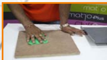
Step 5 : Also SCRATCH plywood Surface
