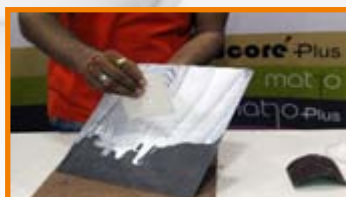
Step 7 : Apply THIN layer of the glue on the surface of the sheet which has been scratch.
