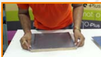
Step 10 : Start pasting sheet from EDGE of the plywood.
