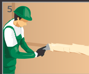
Finishing joint with SHERA jointing solution
